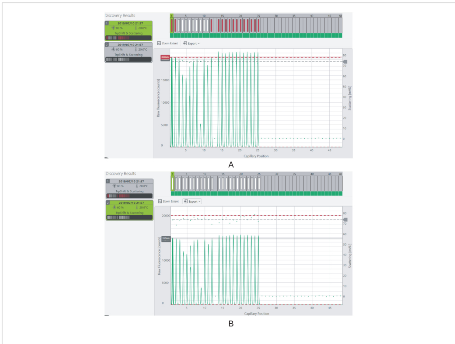
Figure 4: Adjusting the excitation power and fluorescence signal. (A) At 80% excitation power, the fluorescence signal for most of the samples is beyond the saturation limit. (B) The fluorescence signal is reduced to measurable levels by decreasing the excitation power to 60%. Please click here to view a larger version of this figure.
